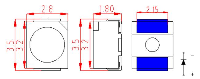
Notice: Tolerance of measurement of Dimension: ±0.2mm
