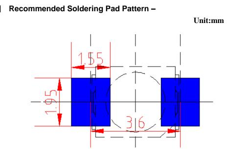
Notice: Tolerance of measurement of Dimension: ±0.2mm
