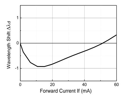
Figure 5. Wavelength Shift VS. Forward Current
