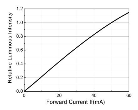
Figure 8. Relative Luminous Intensity VS. Forward Current
