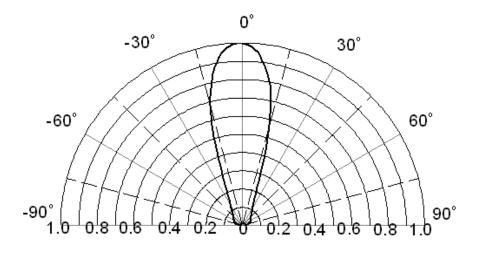
Figure 6. Relative Luminosity VS. View Angle
