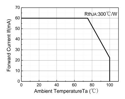
Figure 4. Forward Current VS. Ambient Temperature
