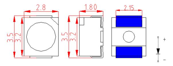
Notice: Tolerance of measurement of Dimension: ±0.2mm
