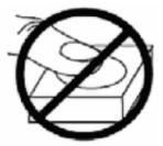
ii. When handling the product with tweezers, LEDs should only be handled from the side and make sure that excessive force is not applied to the resin portion of the product. Failure to comply can cause the resin portion of the product to be cut, chipped, delaminated and/or deformed, and wire to be broken, and thus resulting in catastrophic failure.
