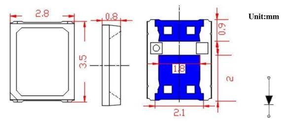
Notice: Tolerance of measurement of Dimension: ±0.2mm
