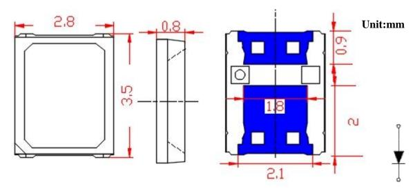
Notice: Tolerance of measurement of Dimension: ±0.2mm
