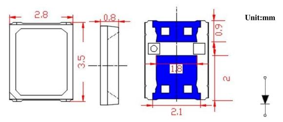
Notice: Tolerance of measurement of Dimension: ±0.2mm
