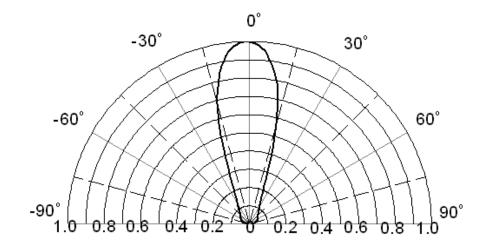
Figure6. Relative Luminosity VS. View Angle
