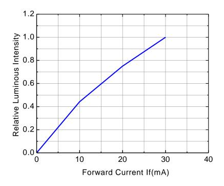
Figure8. Relative Luminous Intensity VS. Forward Current
