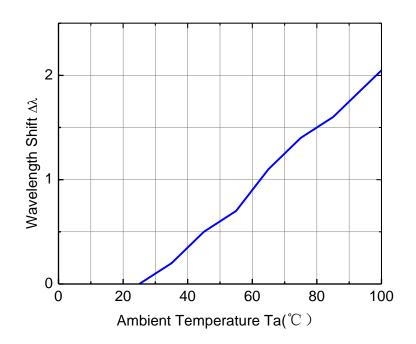
Figure2. Wavelength Shift VS. Ambient Temperature
