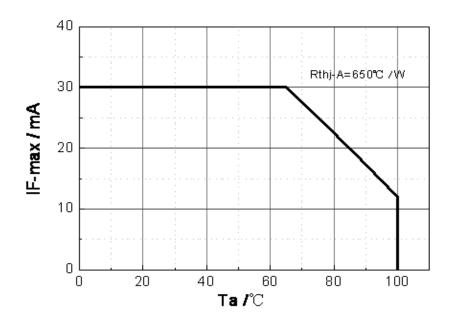
Figure 4. Forward Current VS. Ambient Temperature
